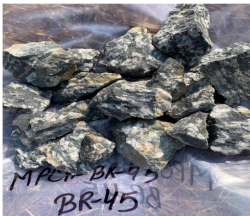
Photo 3: Photograph showing tourmaline, iron oxide in bedrock chip samples MPCH/BR/45.
